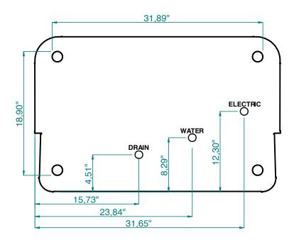
For optimal use of the appliance, check that the water supply pressure exceeds 1 bar (100 kPa) and be less than 6 bar (600 kPa). If the incoming water pressure exceeds 6 bar, we recommend to use a pressure reducer.
