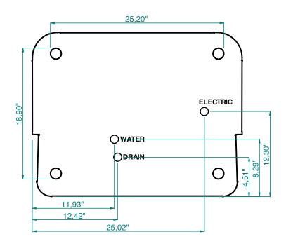
For optimal use of the appliance, check that the water supply pressure exceeds 1 bar (100 kPa) and be less than 6 bar (600 kPa). If the incoming water pressure exceeds 6 bar, we recommend to use a pressure reducer.
